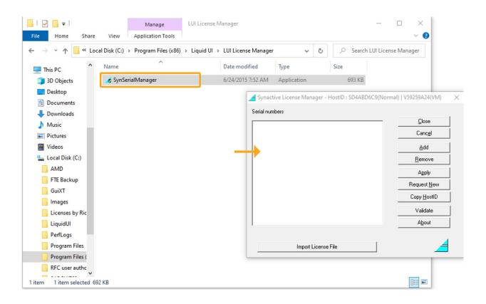
3. In the appeared window, click the **Copy Host ID** button located on the right side of the window. Select the Host ID starting with S and paste the Host ID into a text file. You will need this later on in the process.
